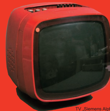
TV „Siemens Alpha 31“, German Federal Republic 1960, Acrylonitrile-butadien-styrene copolymer (ABS)
