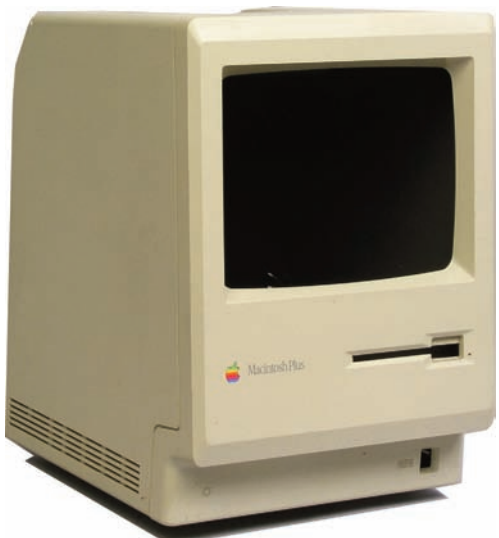
Apple Computer, German Federal Republic 1985, Acrylonitrile-butadiene-styrene copolymer (ABS)
