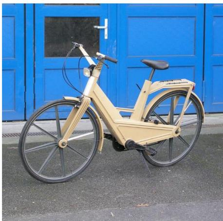
Fahrrad "Itera", Polyamid (PA) 6, Spritzguss
